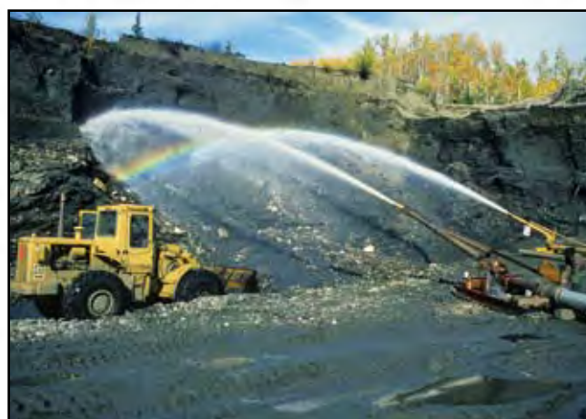
Fig. 7. Hydraulicking at the Levesque Mine in the Klondike goldfield. The water jets are washing out the full thickness of muck and auriferous gravel, and also the top few metres of the altered gold-bearing schist – exposed above the excavator.
